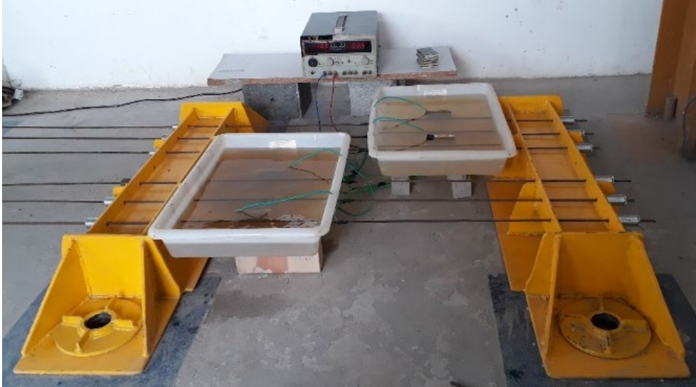
Figure 7 - Corrosion Acceleration Test.
