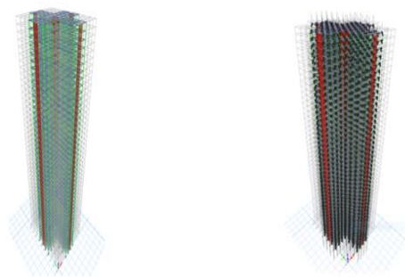
Figure 1-44 Story Linear and Non-Linear Sample Building 3D Models.
